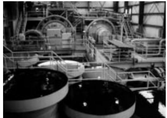
Figure 5. Extracting Gold From the Ore in the Mill Building. Ball and rod mills in background for grinding ore. Columns for recovering gold onto activated carbon are in foreground.
